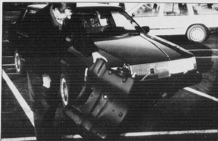
The days of traditional metal fuel tanks could well be increasingly numbered as plastic alternatives such as the one used in the new Volvo 900 series are developed. Neste photo
