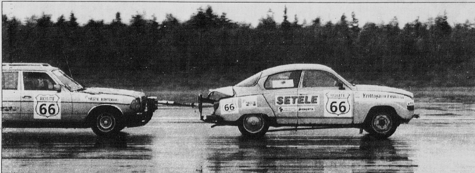
Finnish police testing the harpoon device.
